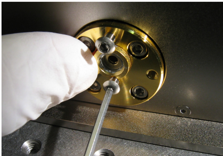
Figure 8-3: Loosen the bottom retaining screw.
