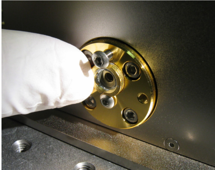
Figure 8-2: Loosen the top retaining screw.
