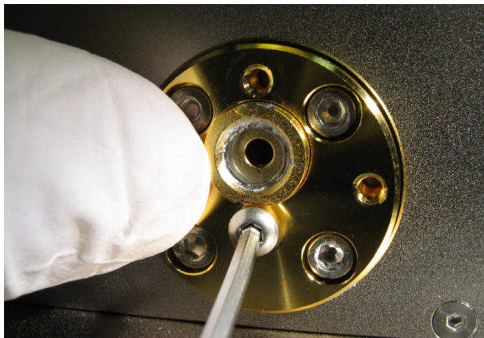
Figure 8-5: Replace the window assembly.
